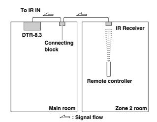
Make the connection as shown below. Do not plug in any equipment to the power outlet until all the connections are complete.
